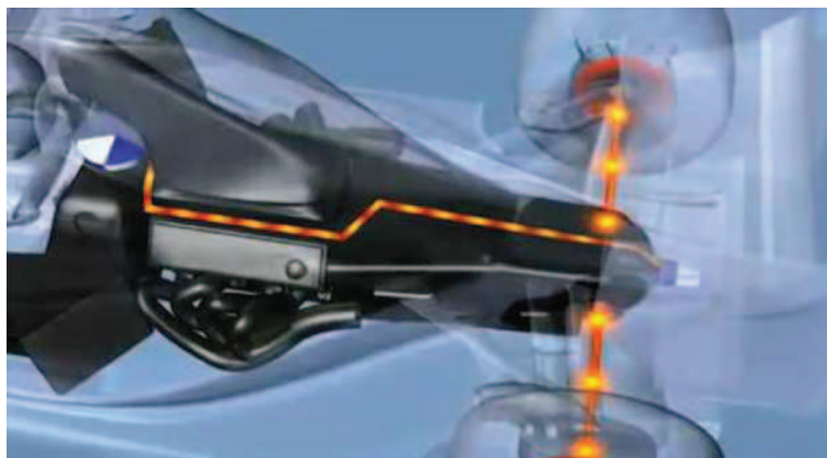
Figure 26: Example of electrical configuration of flywheel-hybrid powertrain (Williams f1)
